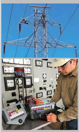
• Low-Pressure Equipment Testing: Testing of relays and circuits, performance testing of high-pressure equipment (e.g., trip CB testing), relay performance adjustment, and relay setting calculations.
